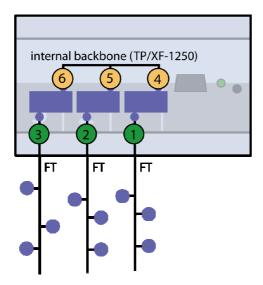
On the attached label, only the external NIDs (number 1-3) are printed. Since the NIDs are organized in a continuous number block, the internal NIDs can be derived by incrementing the numbers printed on the label (number 4-6).
