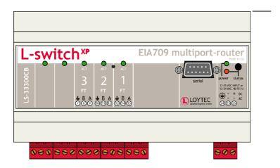
Internally, the device uses 3 individual routers which are connected over an internal(!) TP/XP-1250 backbone.
