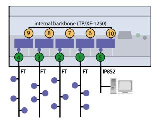
On the attached label, only the external NIDs (number 1-5) are printed. Since the NIDs are organized in a continuous number block, the internal NIDs can be derived by incrementing the numbers printed on the label (number 6-10).
