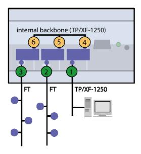
On the attached label, only the external NIDs (number 1-3) are printed. Since the NIDs are organized in a continuous number block, the internal NIDs can be derived by incrementing the numbers printed on the label (number 4-6). Example:
