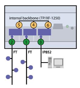
On the attached label, only the external NIDs (number 1-5) are printed. Since the NIDs are organized in a continuous number block, the internal NIDs can be derived by incrementing the numbers printed on the label (number 6-10).
