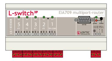
Internally, the device uses 5 individual routers which are connected over an internal(!) TP/XP-1250 backbone.
