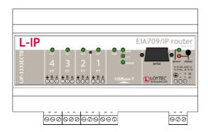
Internally, the device uses 5 individual routers which are connected over a TP/XP-1250 backbone.
